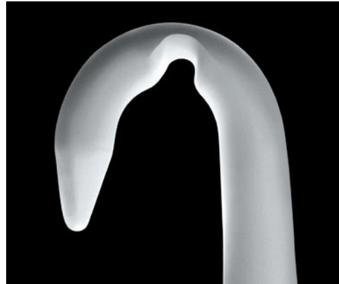
Wear to the inside area of the hook (without coating)
